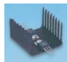
Accepts one or two devices 179-935 H=25, W=42, D=38.0 2 holes dia=4
